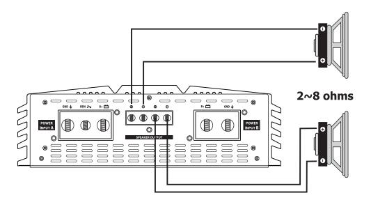
Please note that this unit is a mono block unit and only has one channel Speaker A and Speaker B are just labeled for clear illustration.
